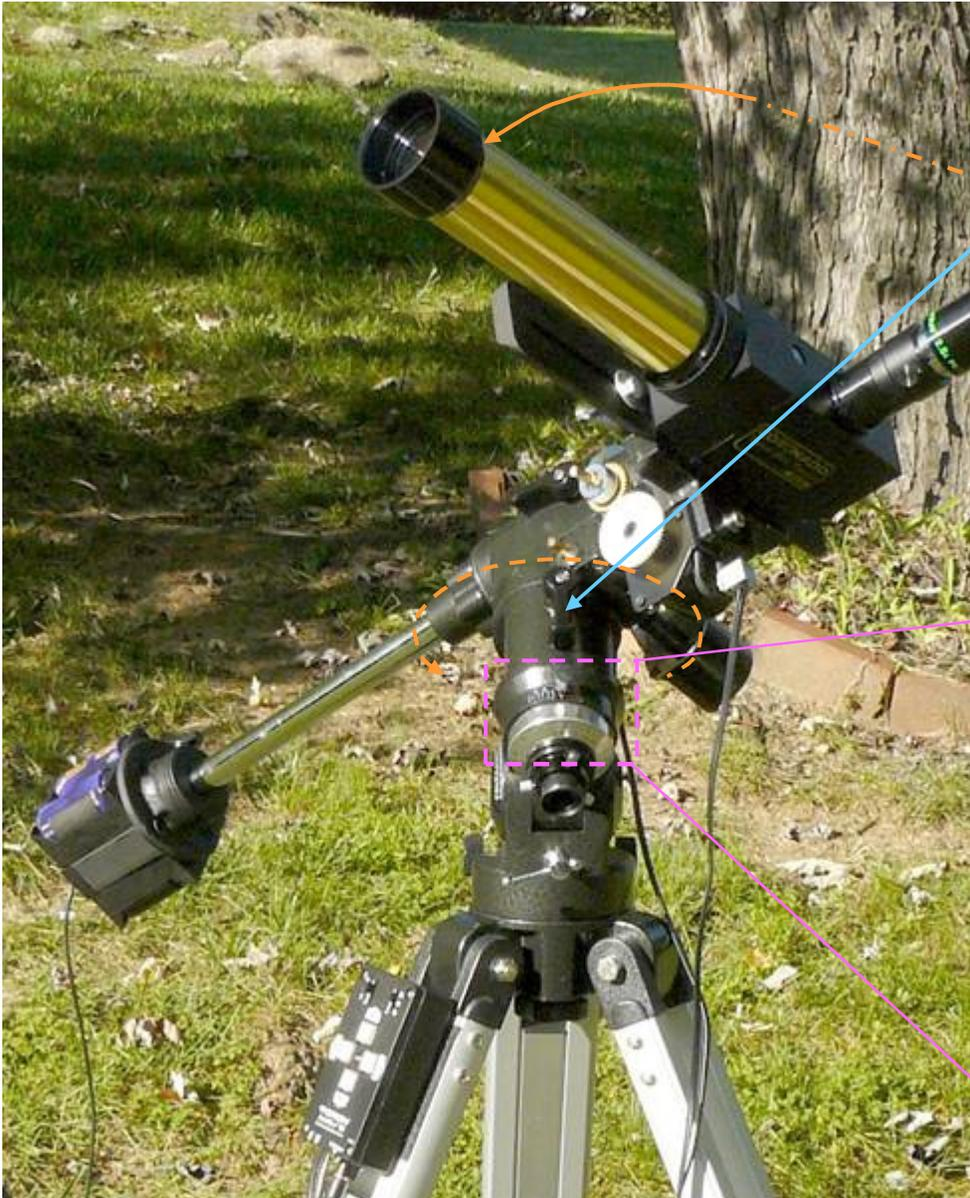
(a) Loosen **RA clutch**, and **push the scope** over so that the RA setting circles indicates the sun's RA position (13:12 in this case). Re-tighten the RA clutch.
