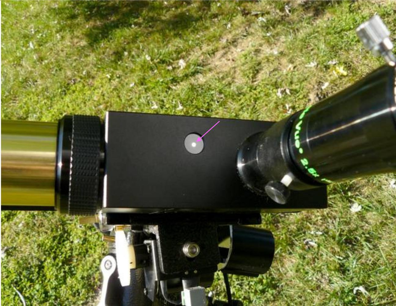
Do the final fine adjustments using the RA and DEC controls to center the sun. If large adjustments are needed, tracking will be less than optimal, so it may be best to start fresh, trying to eliminate errors to minimize inaccuracies.
