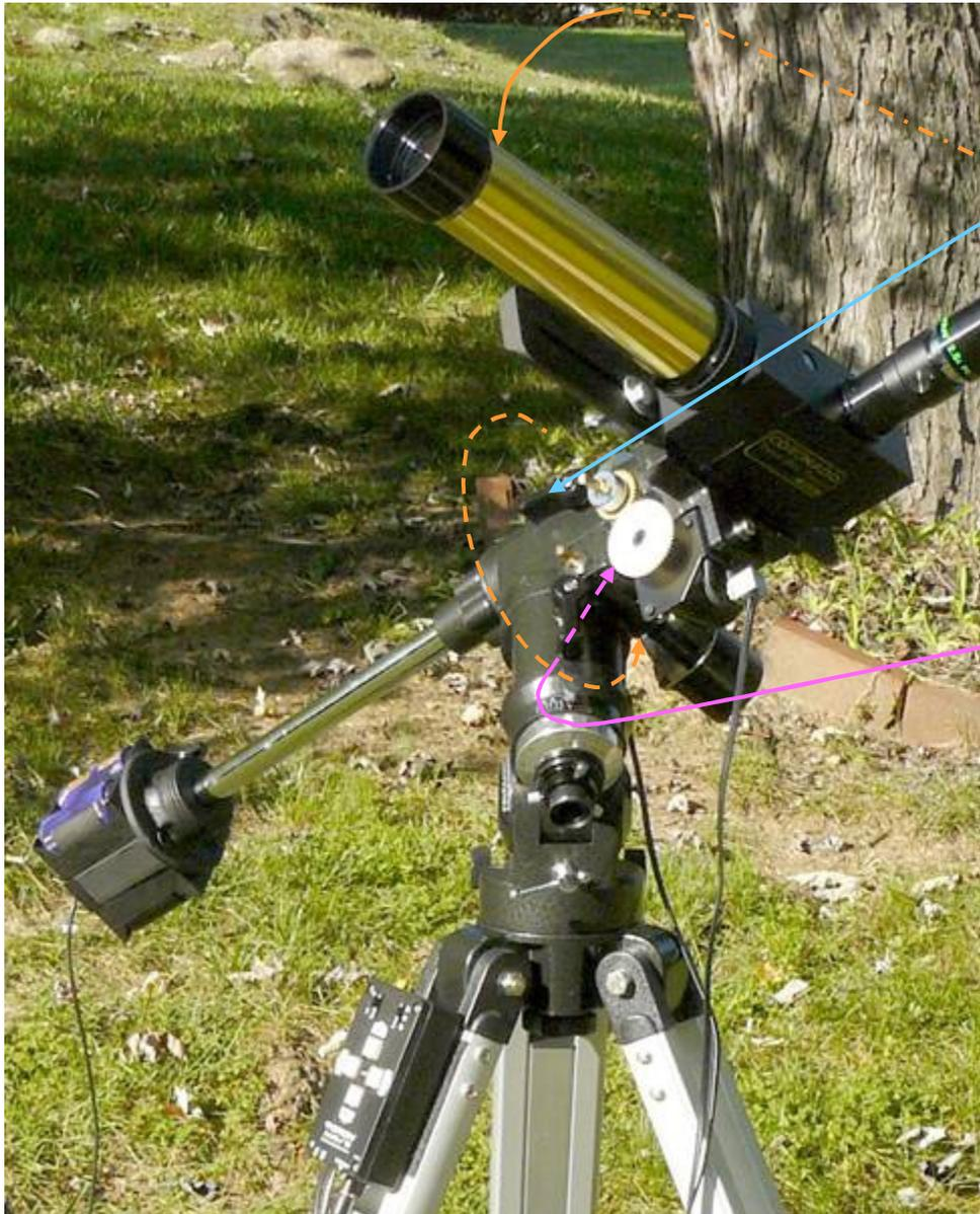
(a) Loosen the **DEC clutch**, and push the scope over so that the DEC setting circles indicate the sun's DEC position ( $-8^\circ$  in this case). Re-tighten the DEC clutch.
